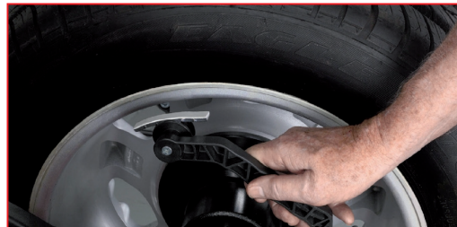
Gauge arm equipped with weight clamp retains the wheel weight in the correct position for weight placement.
